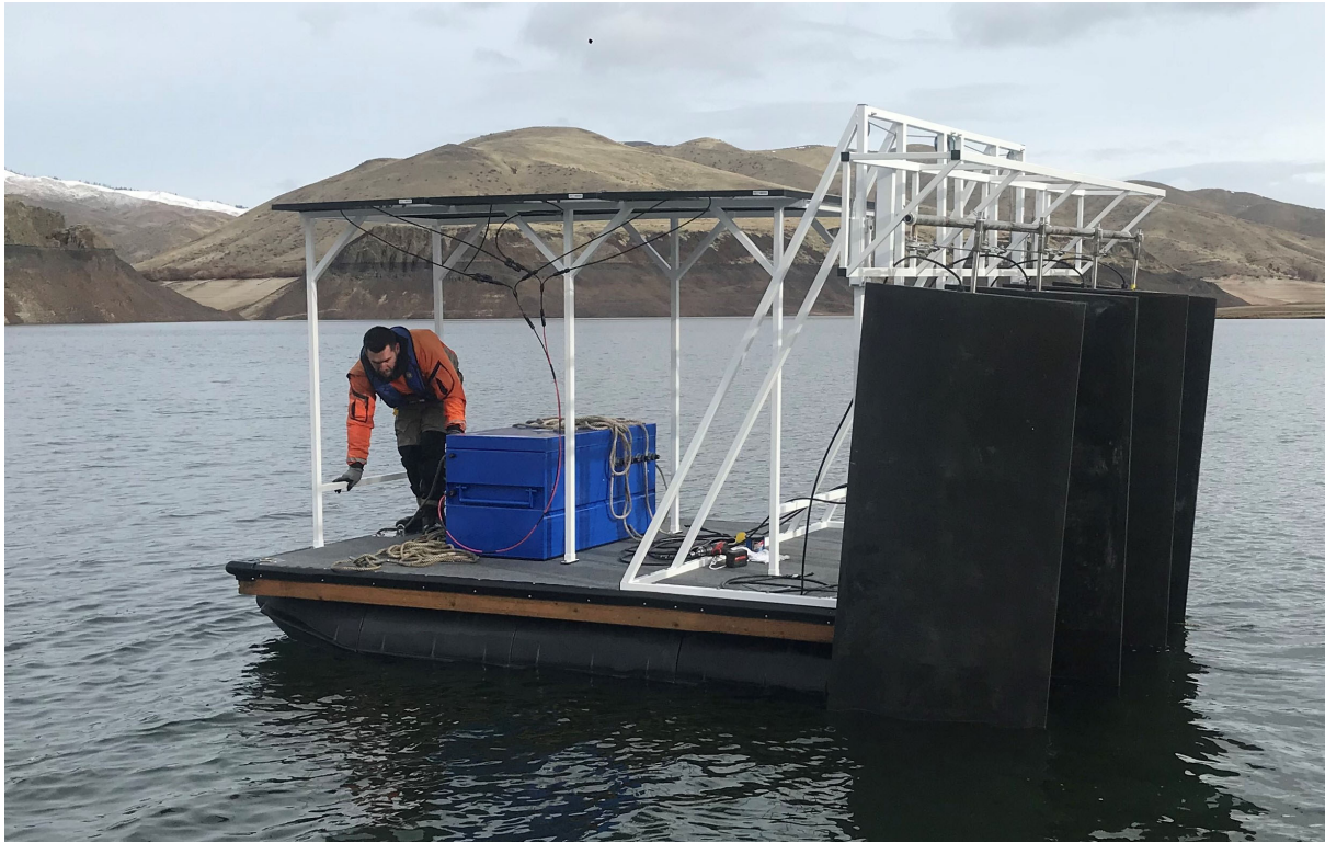
Figure 6-11. Barge Antenna Array
